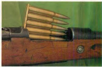
Most military models load through an open bolt with five-round stripper clips.
